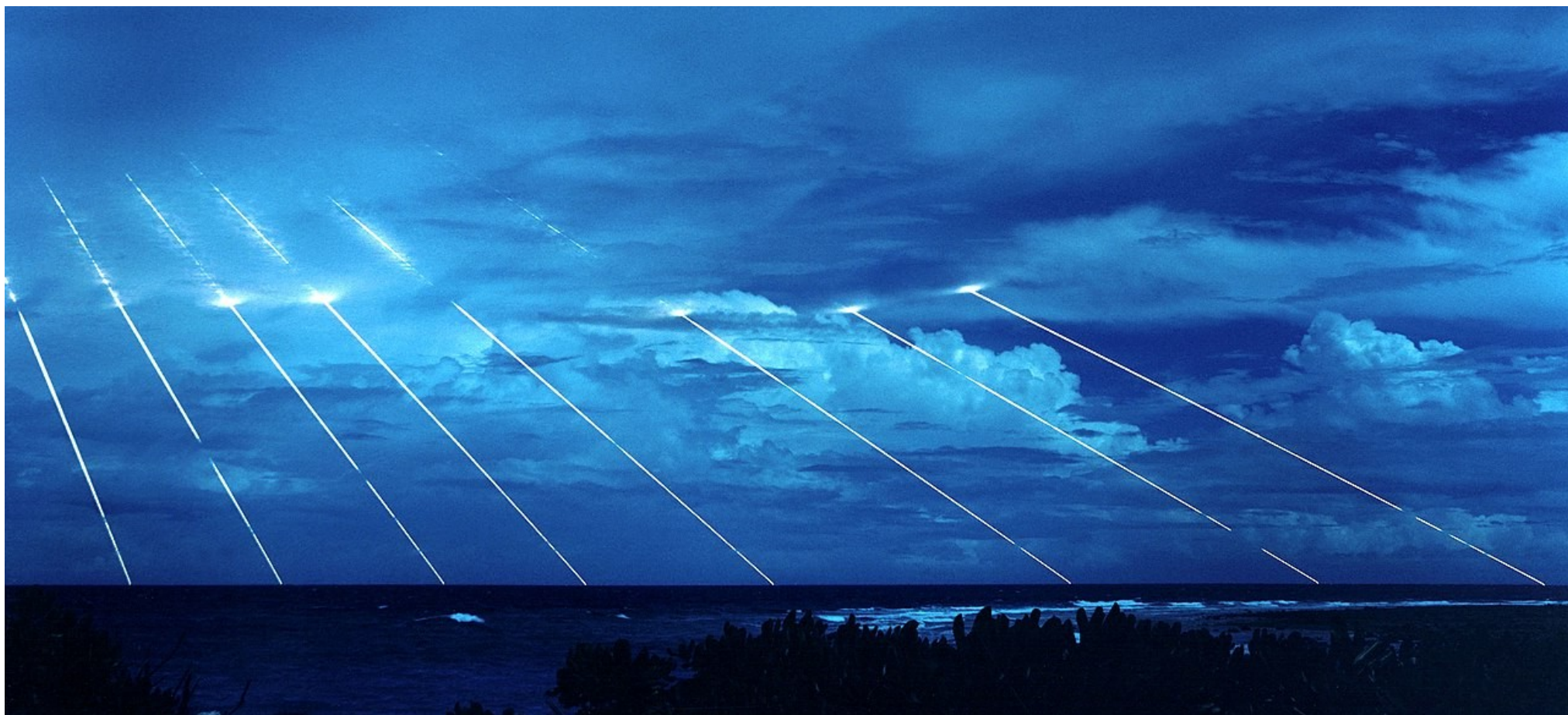
Eight dummy warheads from a single Peacekeeper missile (since retired) during a DoD test.
